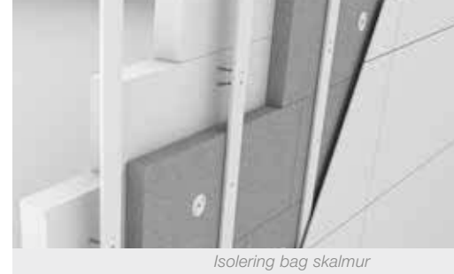
Isolering bag skalmur
