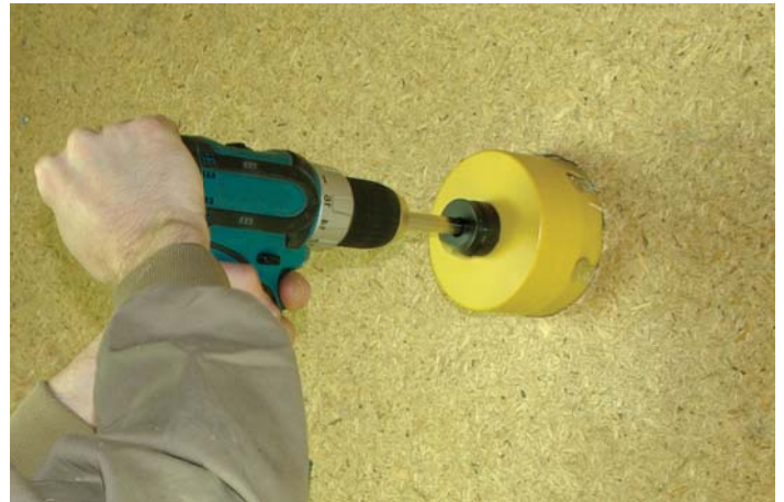
Hole saw with ejection system for injection openings in a variety of materials
