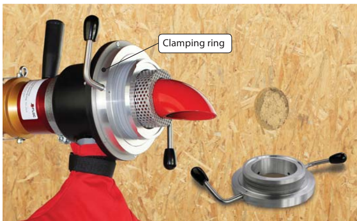
X-Jet with clamping ring
