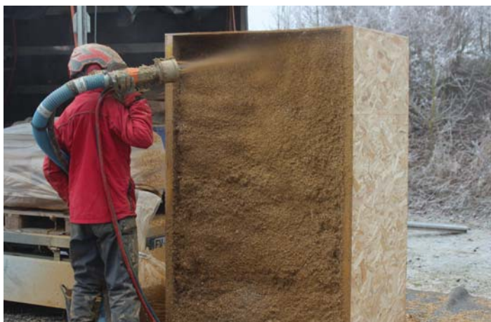
Function test of insulation material and blowing machine
